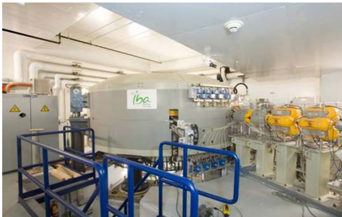
Figure 5. A commercial medical cyclotron, the Proteus 235 by Ion Beam Applications S.A. (IBA). It produces a proton beam with a fixed energy of 250 MeV. The diameter of the accelerator is 2.5 metres, one tenth the size of the CNAO synchrotron ring
